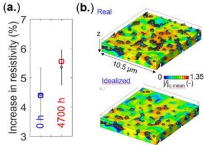
(a) Increase in effective resistivity caused by the Sr-containing phases, in the pristine and aged sample. (b) Current density computed in the pristine sample with (upper) and without (lower) the Sr-containing phase.
